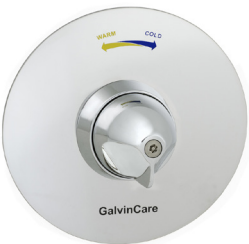
WM-TMVPMSCSUS GalvinCare In-wall Thermostatic Progressive Mixing Valve • Provides state of the art features to comply with healthcare requirements. • The lever handle operates on/off temperature controls • Water is mixed closer to the point of discharge, minimizing stagnant warm water • Smooth internal components and body, reduces scale build-up and bacteria growth.
