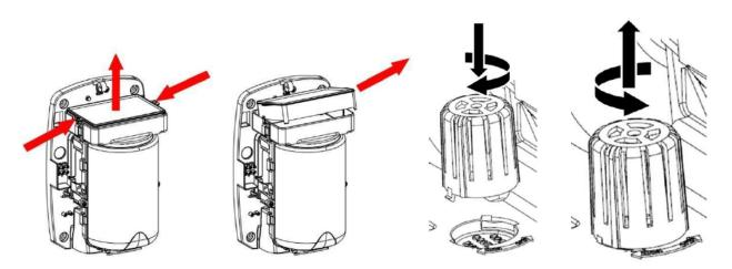
Replace the old filter by pulling from the lateral flaps, as shown on picture.
