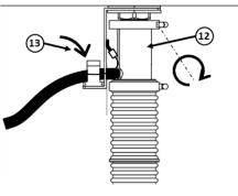
Check the installation so that the IR sensor cables or the ground are not visible, the corrugated tube must completely protect them.
