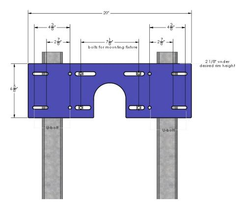
U-bolts, fixture support studs and other hardware supplied by others
